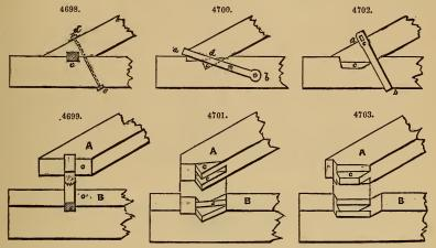
Figs. 4700, 4701, are of a very good form of joint, in which the place of the mortise is supplied by a groove c in the rafter, and the place of the tenon by a tongue d in the tie-beam. As the parts can be all seen they can be more accurately fitted, which is an advantage in heavy work. In Fig. 4700 the mode of securing the joint by a strap *a b* and bolts is shown.
